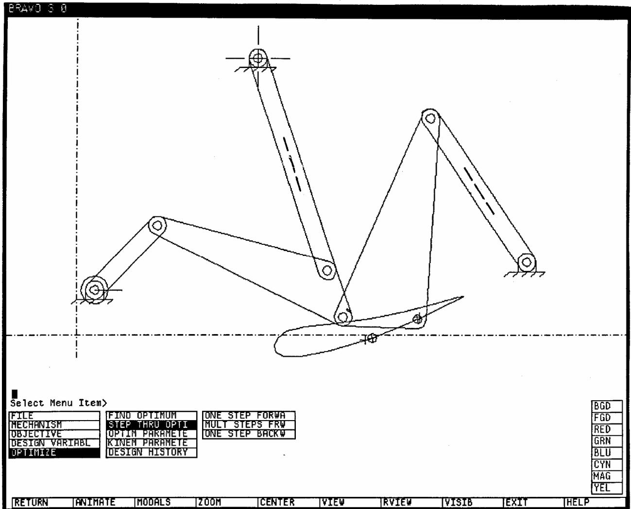
Figure 3: The final mechanism with the objective.
