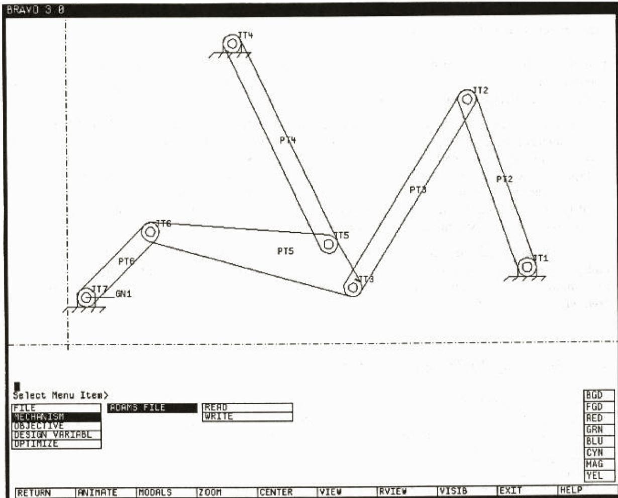
Figure 1: The initial “Stamping Mechanism” and the MSP user interface
