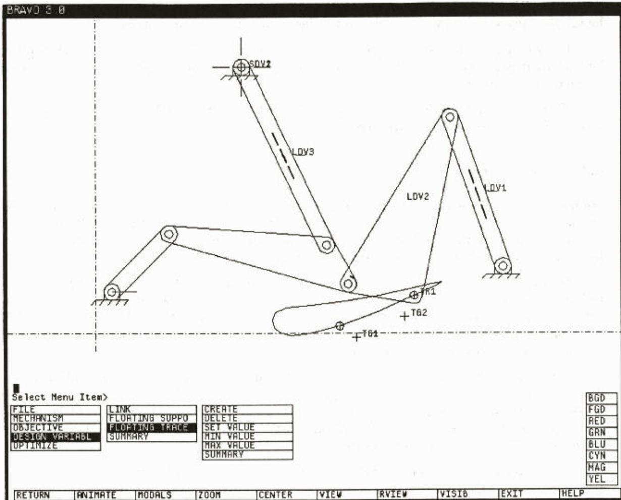
Figure 2: The mechanism with the objective and design variables defined. The objective is the tracer point and two target points. The design variables are denoted by the triple dashed lines.
